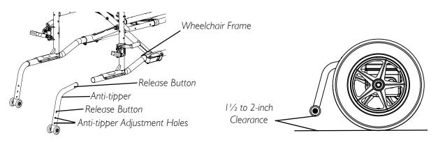
FIGURE 14.1 Installing/Removing/Adjusting Anti-Tippers
